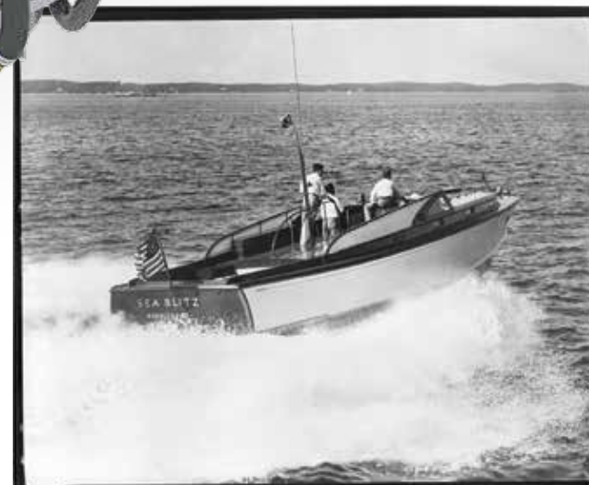
Sea Blitz was the first boat to have a deep-V hull. Shortly after being built, she caught the eye of Dick Bertram, and the hull shape was used in the Bertram 31.
